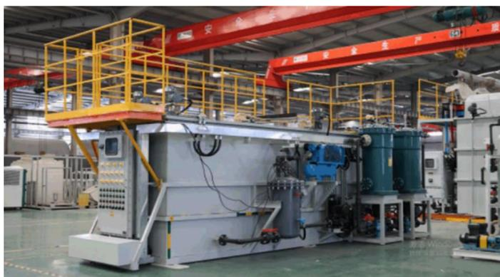
Figure 3. LQF model chemically contaminated water treatment plant
