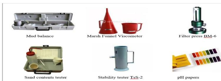
Figure 1. Laboratory equipment for determining the properties of drilling fluid
